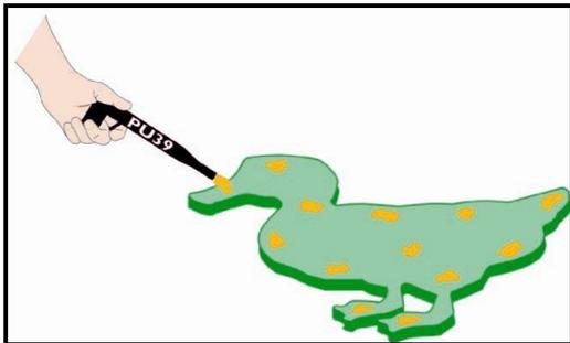
I) Apply dots of Polyurethane glue onto the HEXDALLE® SL element. The HIGH TACK glue is sold in 310-ml cartridges (use with a suitable gun, not supplied).
