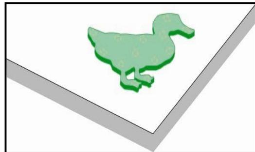
II) Turn the HEXDALLE® SL design over so that the dots of HIGH TACK glue come into contact with the ground. Lightly tap with a rubber mallet or a wooden bar. The HIGH TACK glue sticks instantly.
