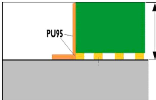
III) Using a brush, apply the polyurethane bonding agent that you use to make your wet floor onto the section of the figurine.
